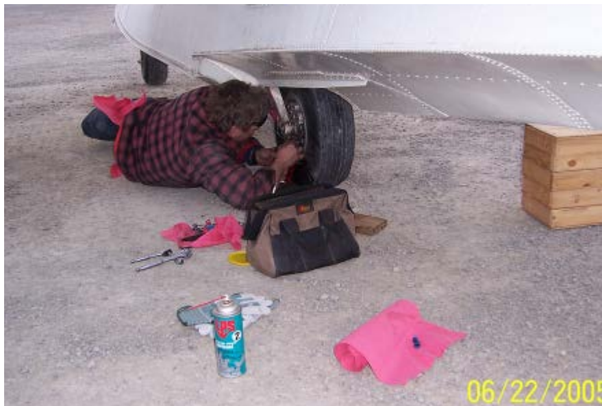
Mechanic working on installing new brakes on N754 in Cambridge Bay, Nunavut, Canada.
